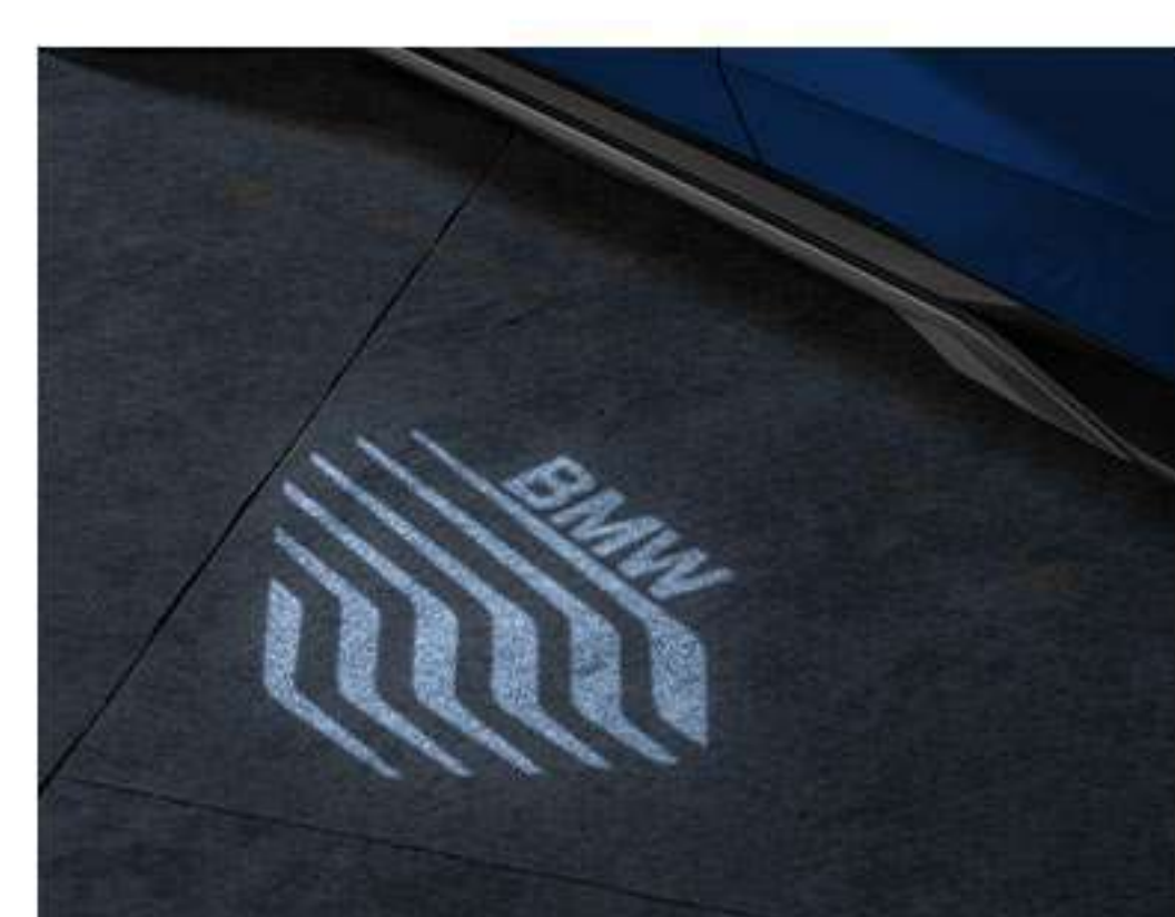
Ambient light package comprises pre-defined selectable light designs in various colors in addition to LED projection with "BMW" logo.
