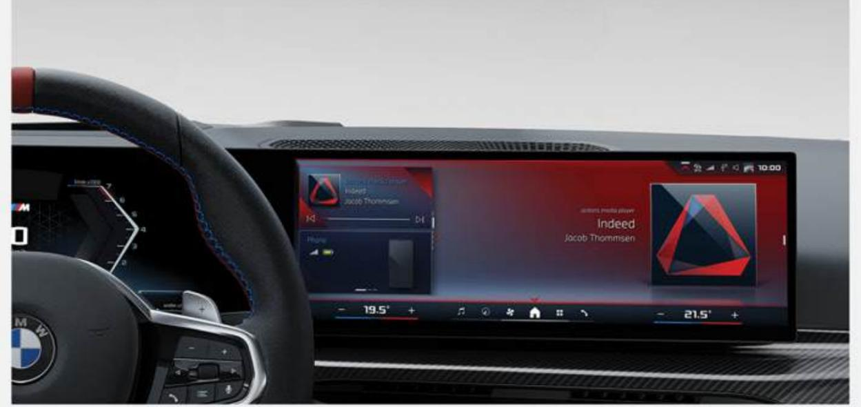
**BMW Live Cockpit Plus:** with navigation function includes a high-quality curved screen display consisting of a high-resolution Display cluster consisting of a fully digital 12.3" instrument display and a high-resolution 14.9" control display.
