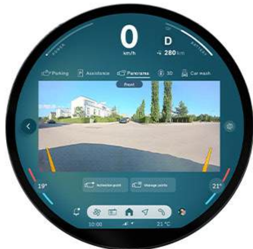
Parking Assistant Plus: Visual parking aid featuring Surround View cameras, Top View, Panoramic View and 3D View makes parallel and perpendicular parking on the road easier. The system completely takes over the steering, the accelerator, and the transmission. (Only for S & JCW Engines).
