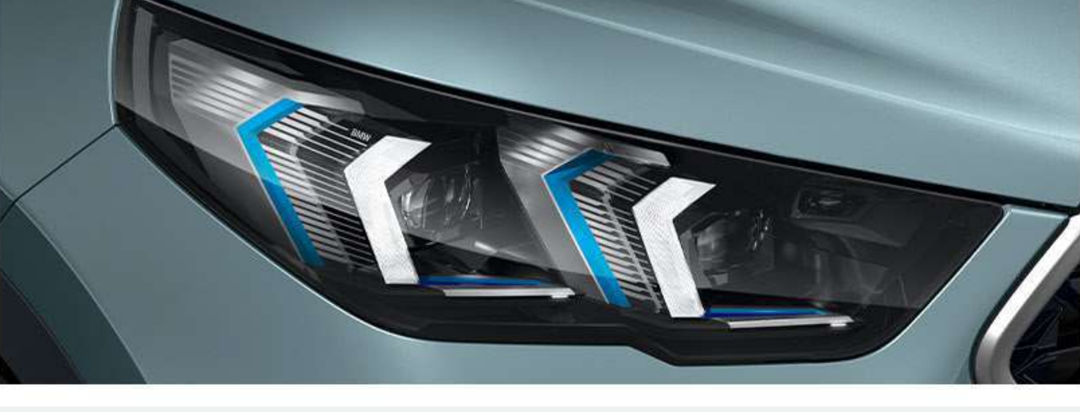
Adaptive LED Headlights with cornering lights offer a bright and efficient bi-LED light for low beam and high beam featuring BMW Selective Beam and High Beam Assistance.
