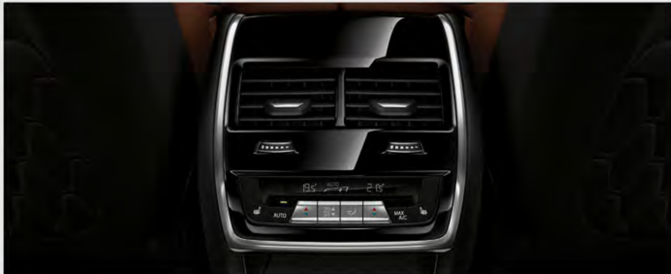
4-Zone Automatic Air Conditioning: includes separate temperature control for driver, front passenger and also left and right rear passengers.
