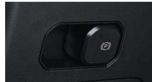
Electronic parking brake with auto-hold function
