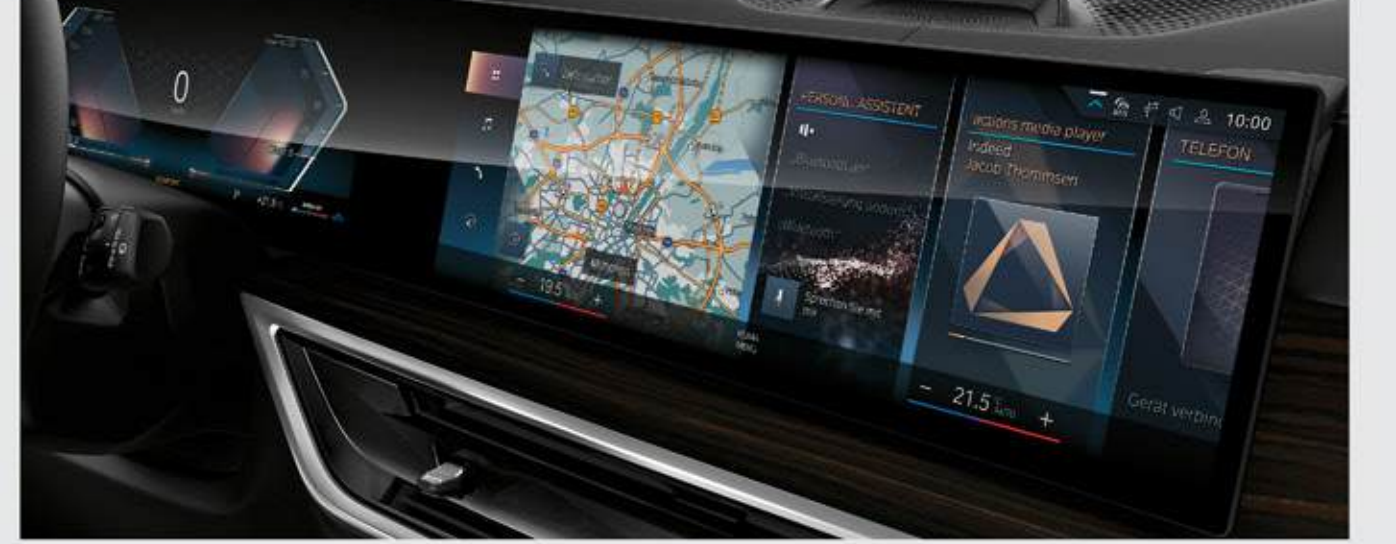
BMW Live Cockpit Professional: a Curved Display that consists of a high-resolution 12.3" instrument display and a touch optimized 14.9" control display with BMW OS 8.5.
