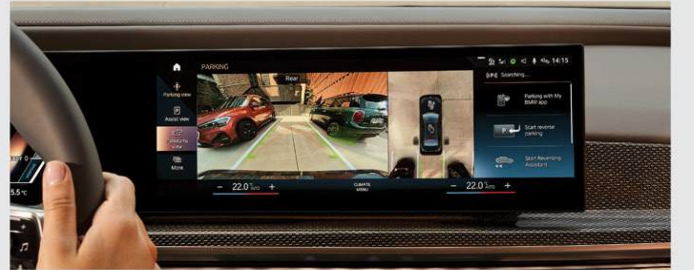
Parking Assistant Plus: Visual parking aid featuring surround view cameras, Top View, Panoramic View and 3D View makes parallel and perpendicular parking to the road easier. The system completely takes over the steering, the accelerator, and the transmission.
