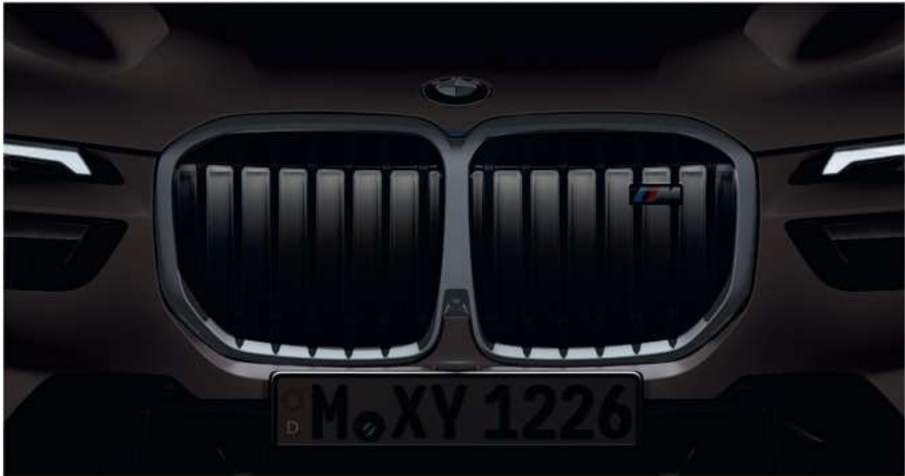
BMW "Iconic Glow" active kidney grille: highlighting of BMW radiator grille by innovative LED fibre optical technology (in white). "Active" indicates the opening and closing of the air vents to actively regulate the airstream. They close for increased aerodynamics and open if the cooling demand for the engine increases.
