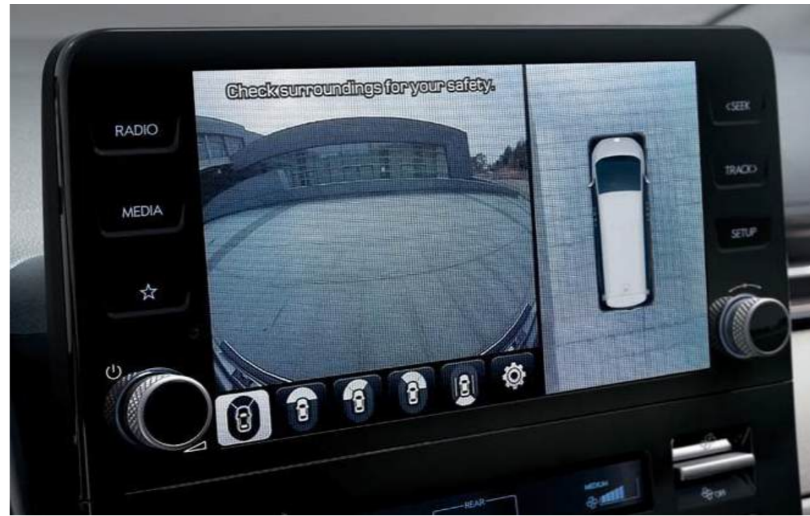
Surround View Monitor Surround View Monitor displays video of the situation around the vehicle for safe parking.
